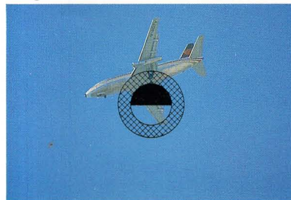
Conventional split-image rangefinder
