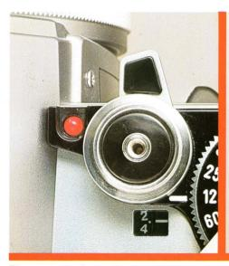
Electronically Controlled Self-Timer After pushing the self-timer lever forward, the self-timer can be activated by the shutter release button. The shutter will be released after a 10-second lag and a red LED lamp will flash to indicate its operation.
