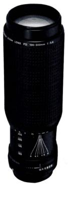
SPECIFICATIONS Type: Tele-zoom w/Macro Construction: 15 elements in 9 groups Angle of view: 24°-8°15' Minimum Aperture: f32 **Closest Focusing Distance:** Normal-2m (6' 63/4") Macro-1m (3' 35/16") Lenshood: Optional, BT-58 (C44-5802) Length: 172mm (613/16") Weight: 705g (1 lb., 93/4 oz.) Cap: C58 (CG2-0072) Case: Optional, LH-C21 (C47-1081), LS-B21 (C47-0956) Function: Auto aperture, full aperture metering, AE operation with all Canon Automatic SLR cameras Coating: Super Spectra
