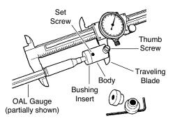
When using the OAL (Over-All Length) Gauge and Bullet Comparator in combination, always attach the Comparator Body to the "traveling" blade - in the off-center position then measure using the configuration shown in the illustration. This method will align the OAL Gauge parallel to your caliper. For all other uses, the Comparator Body may be attached to either blade in the "on-center" position.
