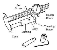
Now, open the caliper and center the case shoulder into the Bushing. Bring the caliper blade to rest on the case head and rotate the case as you remove slack, then take a reading. Be consistent! Most handloaders prefer to carefully "zero" the caliper's indicator on the longest (fire-formed) case. This allows them to gauge the headspace variations from this fire-formed (maximum) case dimension.
