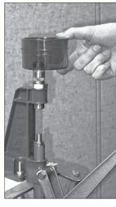
Install the case catcher over the guide sleeve. If you own a Pro 1000 or Loadmaster the quide sleeve is sized to accept the case feed tubes.
