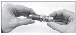
**C** Raise the ram with push pin to the top of stroke. Screw the Factory Crimp Die into the press until the push pin enters the Factory Crimp Die-a minimum of 1/4 inch. (This will push the case completely through the carbide insert.)
