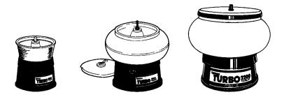
*Cover Removal:* Turbo Pop Top, 600, 1200 – To remove the cover, unscrew the rubber-coated nut in the center of the bowl cover. With the nut removed, the top cover will lift off. Note: It is essential that the nut be tightened securely so that the cover will not vibrate loose. When reinstalling the cover, tighten the nut until the rubber begins to bulge (see sketch.)
