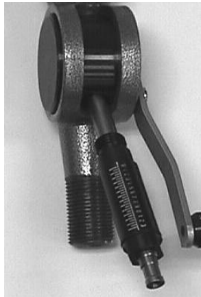
Attaching Micrometer body to Measuring screw
