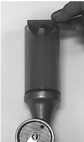
Installing powder baffle
