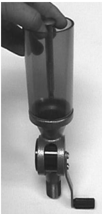
Inserting Rifle Measuring Screw Into measuring Cylinder
