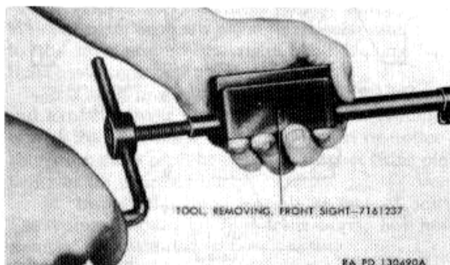
Figure 63. Removing front sight.
