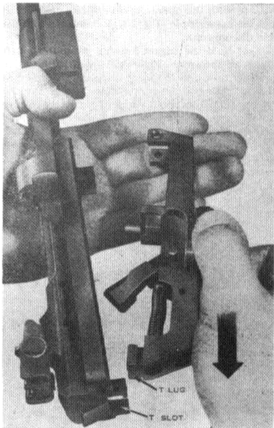
Figure 16. Replacing the trigger housing group.
