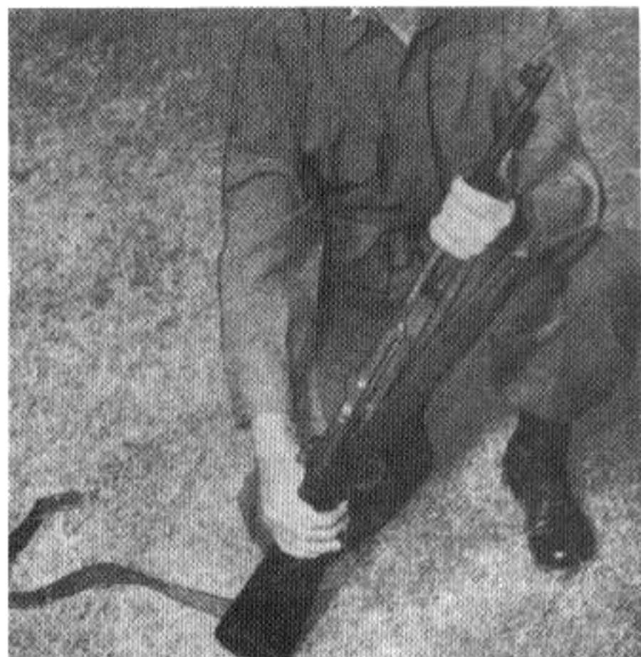
Figure 18. Assembling the stock group and the barrel and receiver group.
