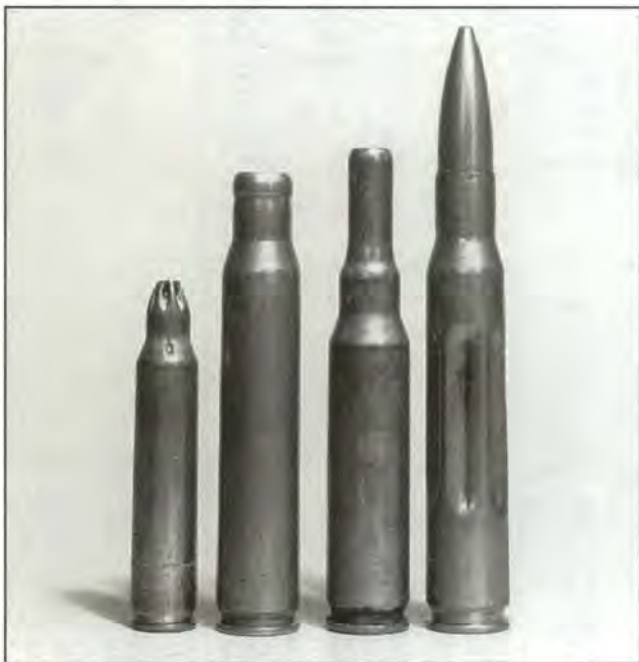
Blanks are made of substandard brass and often contain flaws, like the 223 case with the star crimp. This crimp, as with the flutes on the sides of the 30-06 dummy round, weakens the metal. These cases would likely split in the reloading die or in the next firing. In short, don't try to use brass from blanks, grenade launching or dummy rounds.
