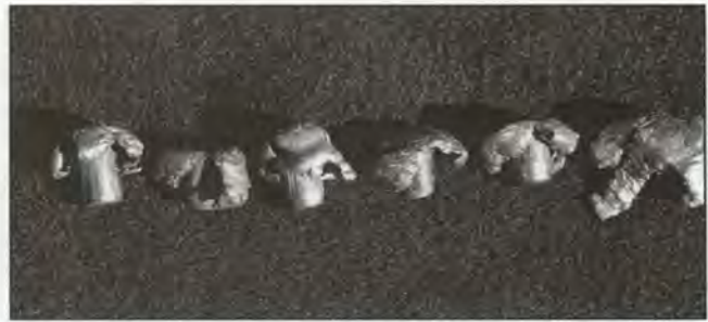
A group of 30-caliber 180-grain bullets recovered from big game. With each bullet, major bones were hit and adequate penetration realized at ranges from 75 – 250 yards. These are what well-constructed bullets should look like.
