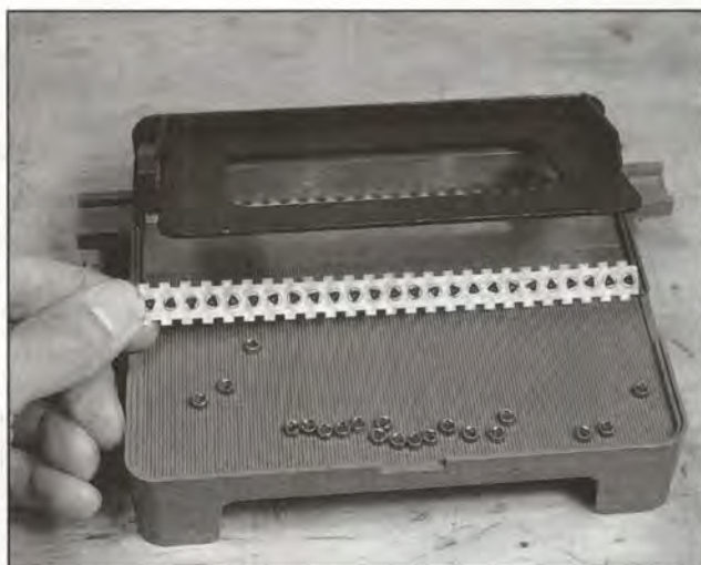
RCBS APS Primer Strip loader tool loads 25 primers in a strip in just seconds.
