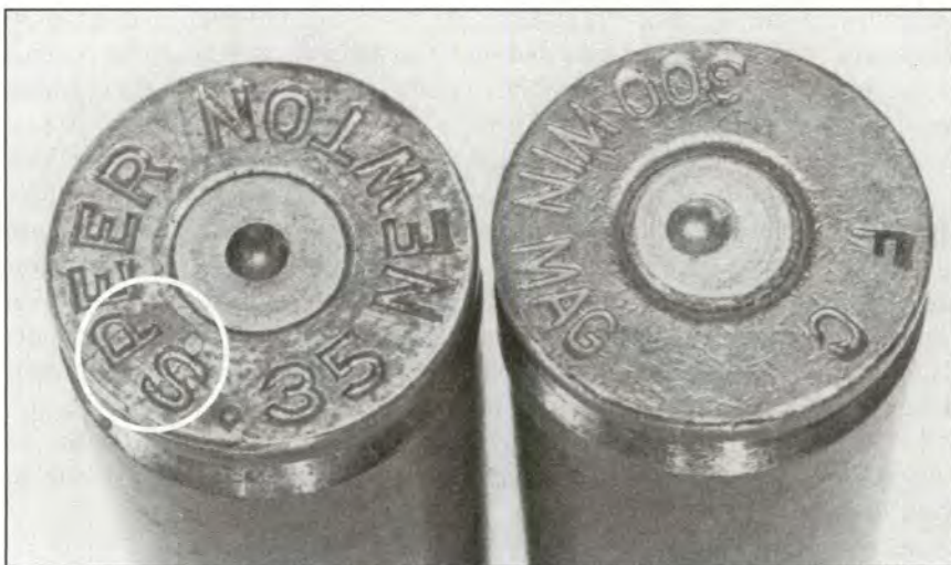
Was the flat primer on the left a result of high pressure or being too soft? The answer is likely high pressure since the case head also flowed into the extractor groove (circled).
