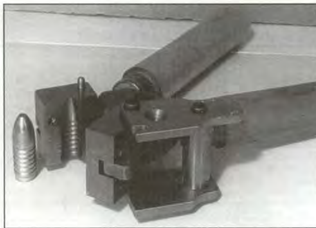
This nose-pour mould from Colorado Shooter's Supply delivers a bullet with a perfect base since the cut-off is at the bullet nose.
