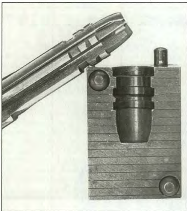
The mould cavity is given final form with a cherry, a reaming tool in the form of the bullet.
