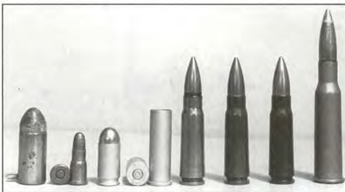
All of these rounds are non-reloadable for a variety of reasons. Left to right: The 12mm pinfire could theoretically be reloaded, but no components are available; tiny 230 Morris used a smaller than standard primer (not available), but new cases can be formed from cut-down 22 Hornets; aluminum and steel cases are for one-time use. "Posts" in the aluminum CCI Berdan primer pockets are battered in the first firing. The steel 7.62x39mm and 7.62x54mm Russian military cases are Berdan-primed and difficult to decap, but it can be done. The two darker cases are lacquer coated to make them function through autoloaders. This coating will likely come off in your reloading dies. In short, it's not worth the effort with Boxer brass cases becoming commonly available.
