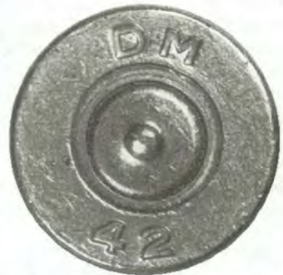
(Above and below) Military ammunition generally has the primer swaged in the case with a primer crimp, which makes first-time removal a little difficult. Once the crimp is removed, however, there is no further problem.
