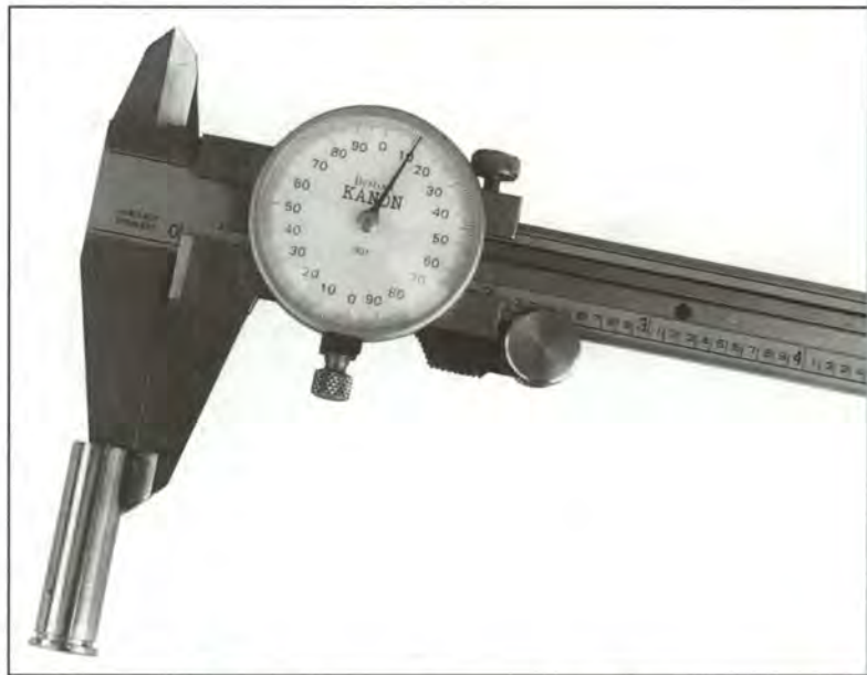
Sorting brass by neck thickness helps ensure the bullet be well-centered in the case and crimping more uniform.
