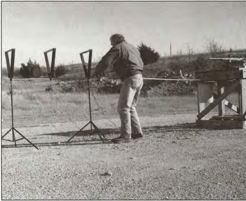
From the muzzle to the chronograph's first screen should be approximately ten feet regardless of whether rifle or handgun is used. Oehler recommends three feet for chronographing shotgun loads.
