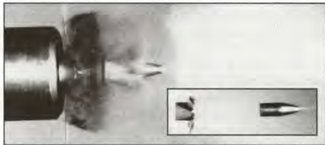
Exterior ballistics involves all that happens to the bullet from muzzle to target. Here's a Remington Accelerator leaving the muzzle at 4080 fps, and the sabot and bullet 18 inches downrange.
