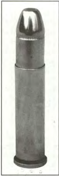
A good example of a perfectly belled case where the sides are not excessively bent away from the bullet.
