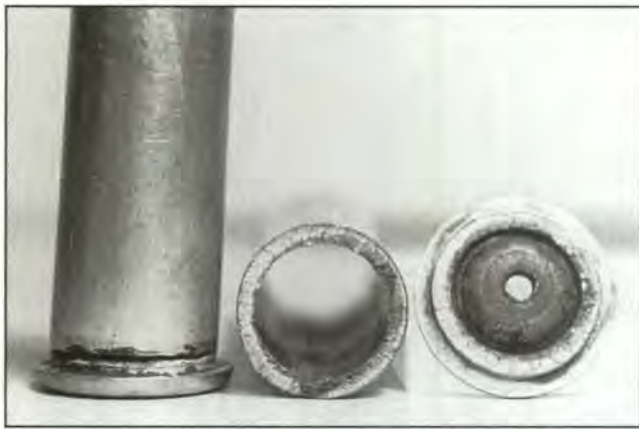
The REM-UMC case on the left suffered near total separation due to mercury contamination. This same factor caused the one on the right to pull apart in the resizing die.
