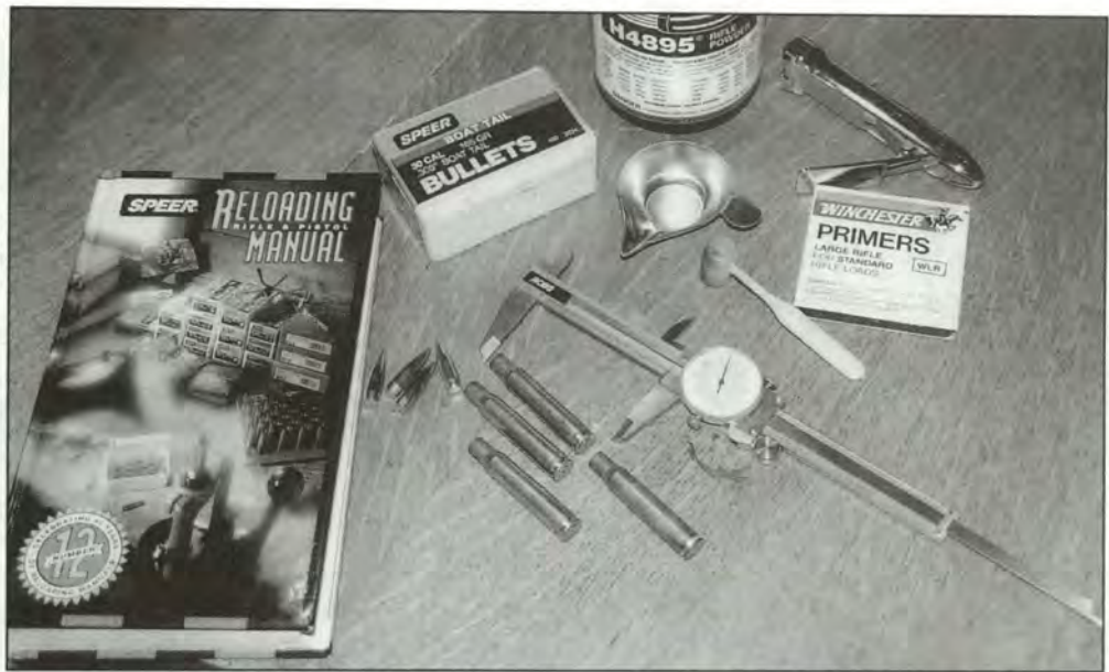
Quality components are essential to loading accurate ammunition. Measure your cases with a dial caliper, round up quality bullets, powder, primers and tools, and rely on your loading manual.
