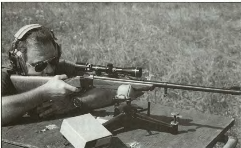
Author chronographing 375 H&H Magnum loads using a P.A.C.T. chronograph, an excellent instrument.
