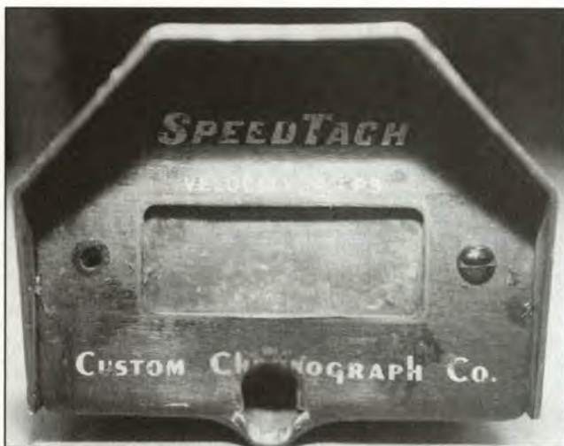
This SpeedTach was dealt a fatal blow by a cast 9mm bullet, something to consider when using an "up front"-type instrument.
