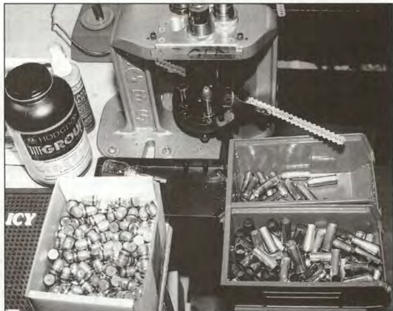
Everything is arranged for speed (RCBS Case Slick really helps on big cases even though carbide dies are used).
