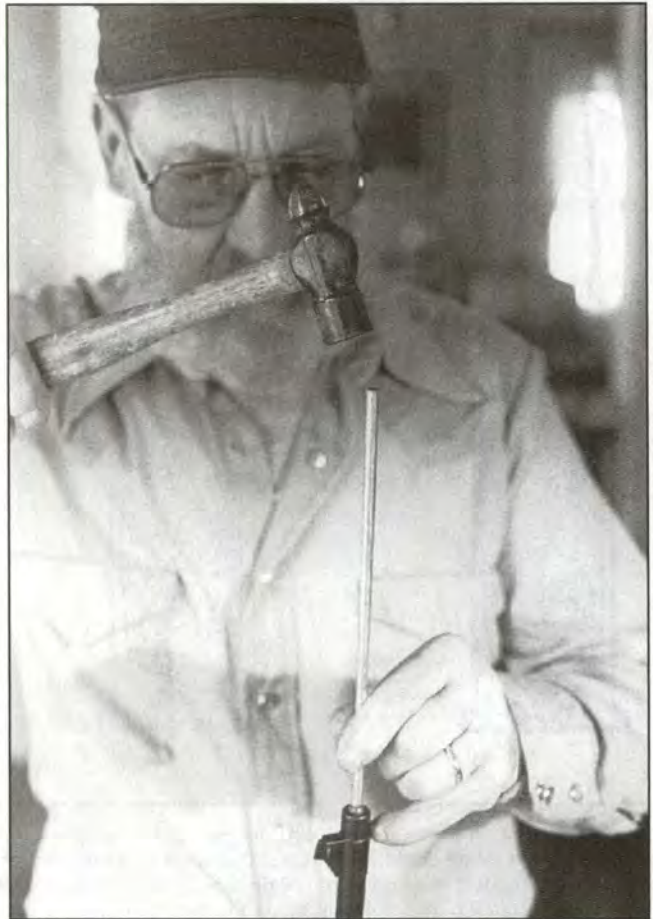
(Above and right) Slugging the bore consists of carefully driving a small, soft pure lead slug down the barrel. If done from both ends, the two slugs can be compared for tight and loose spots in the barrel.
