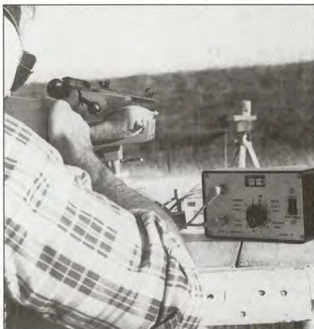
Author's first chronograph was this Oehler Model 12 of 1980 vintage. Perhaps a little slow by contemporary standards, it was affordable and worked well.
