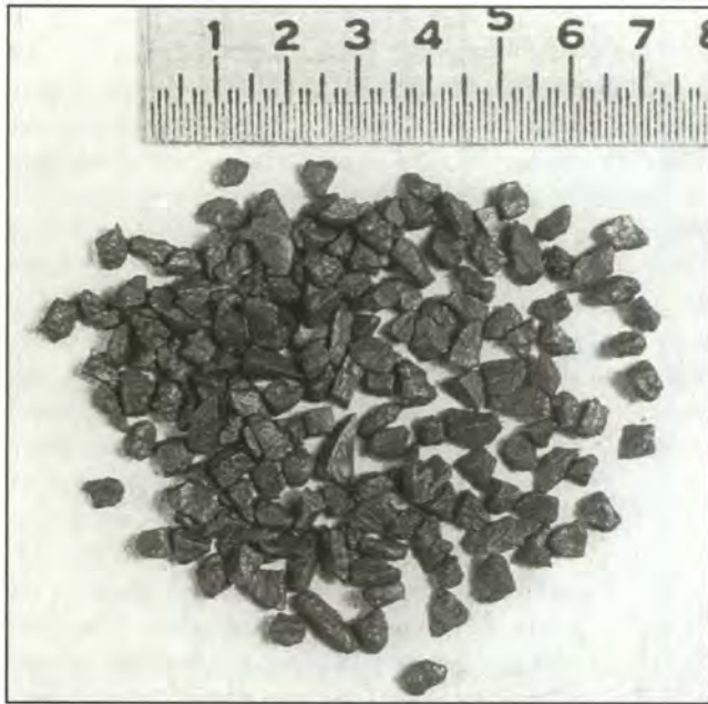
Ffg blackpowder is a fairly coarse-grained propellant. The scale above is 1 inch divided into hundredths.
