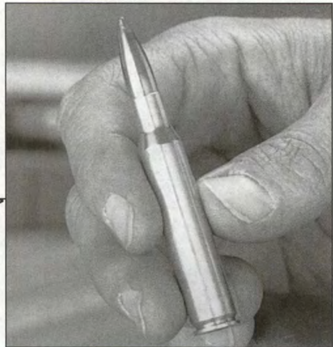
Step 19 - The Loaded Round: After wiping off any sizing lube, the first loaded cartridge is ready to be fired.
