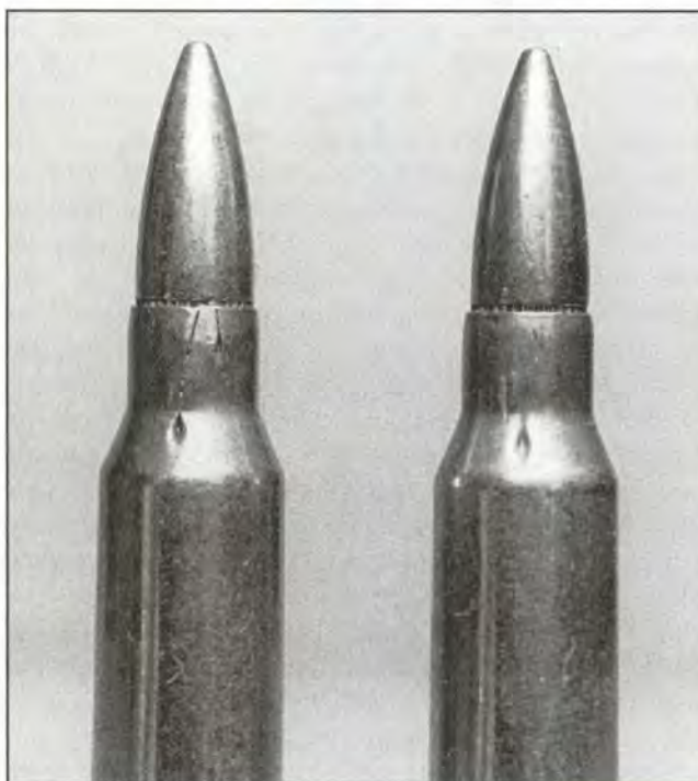
(Above) Manufacturing defects, in this instance what appears to be poor brass, resulted in split necks in these 223 military cartridges.
