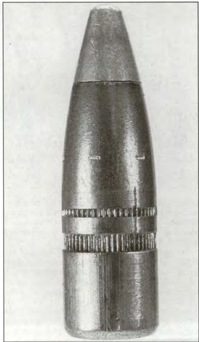
Winchester's Silvertip hunting bullet features a thin aluminum jacket over the lead point. This allows good expansion, but prevents the bullet from getting nicked and dented as the cartridge is fed through the magazine.
