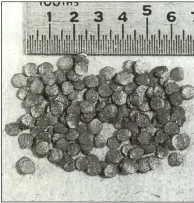
Alliant Unique powder is a powerful, fast-burning double-base propellant used in pistol and light rifle loads. It is a fine, flake powder that has been made for nearly a century.
