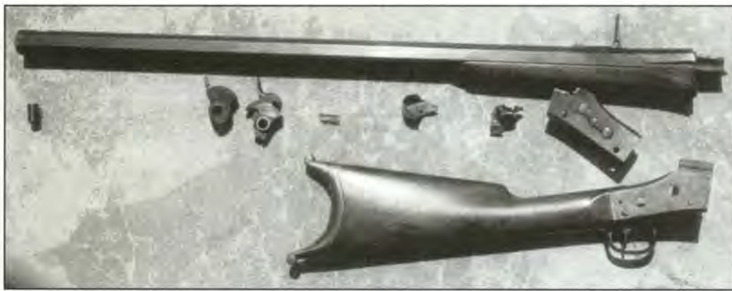
The sad end of a fine old rifle—accidentally overloaded with a double charge. (Photo courtesy of Tom Trevor)
