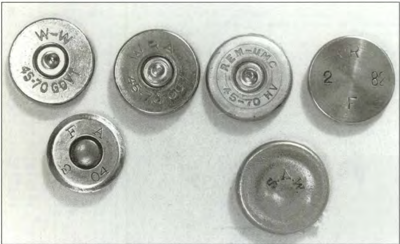
What headstamps tell you. Commercial ammunition is marked with the caliber and name of the manufacturer, at least in this country. Military ammunition is usually stamped with the code of the arsenal or manufacturer and the date of manufacture. Top row, left to right: a 45-70 current headstamp, pre-WWII commercial Winchester and Remington headstamps (good candidates for being mercuric primed), and an inside-primed military centerfire from the 1880s. R indicates a rifle load, F is the code of Frankford Arsenal, 2 82 indicates it was loaded in February, 1882. Bottom row: a 30-40 Frankford Arsenal round loaded February, 1904, and a Spencer 52-caliber rimfire made by the Sage Ammunition Works.
