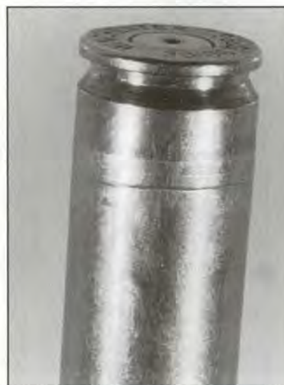
Stretch marks and the crack on this case are indicative of excessive headspace. (Photo courtesy Speer.)
