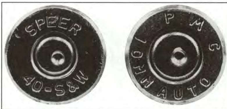
Even though the 40 S&W and the 10mm Auto have the same case and bullet diameters, they use different size primers.
