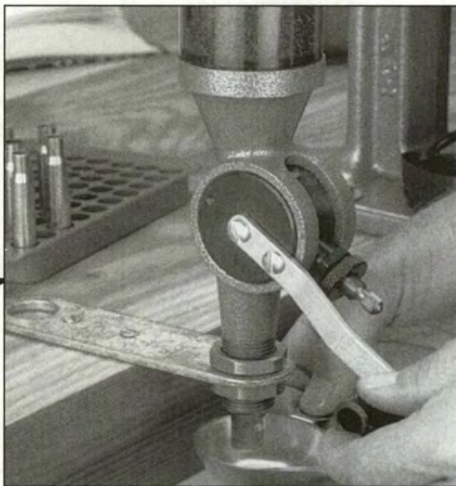
Step 14 - Powder Charging (C): Another method of charging is to use the powder measure. It dispenses a precise, uniform charge with each crank of the handle, thereby speeding up the process. Use the reloading scale to adjust the powder measure until it throws several identical charges. Then, weigh about every ten charges to recheck the weight.
