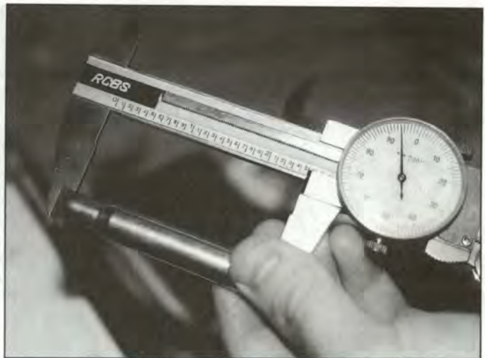
Especially with rifle cases, it is critical to check their length before reloading, to see that they will chamber properly. Another essential process for producing accurate loads is to clean and prepare cases. If it is necessary to trim a case, the mouth should be prepared by removing any sharp edges.
