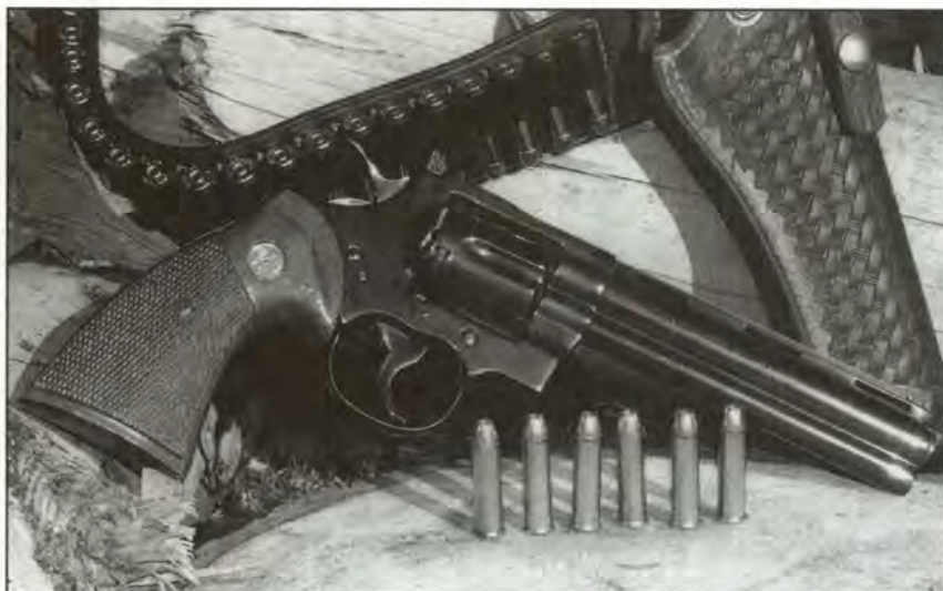
Colt Python in 357 Magnum, shown here with author's handloads topped by 158-grain Hornady XTPs, a bullet easily capable of bringing down deer-sized game.
