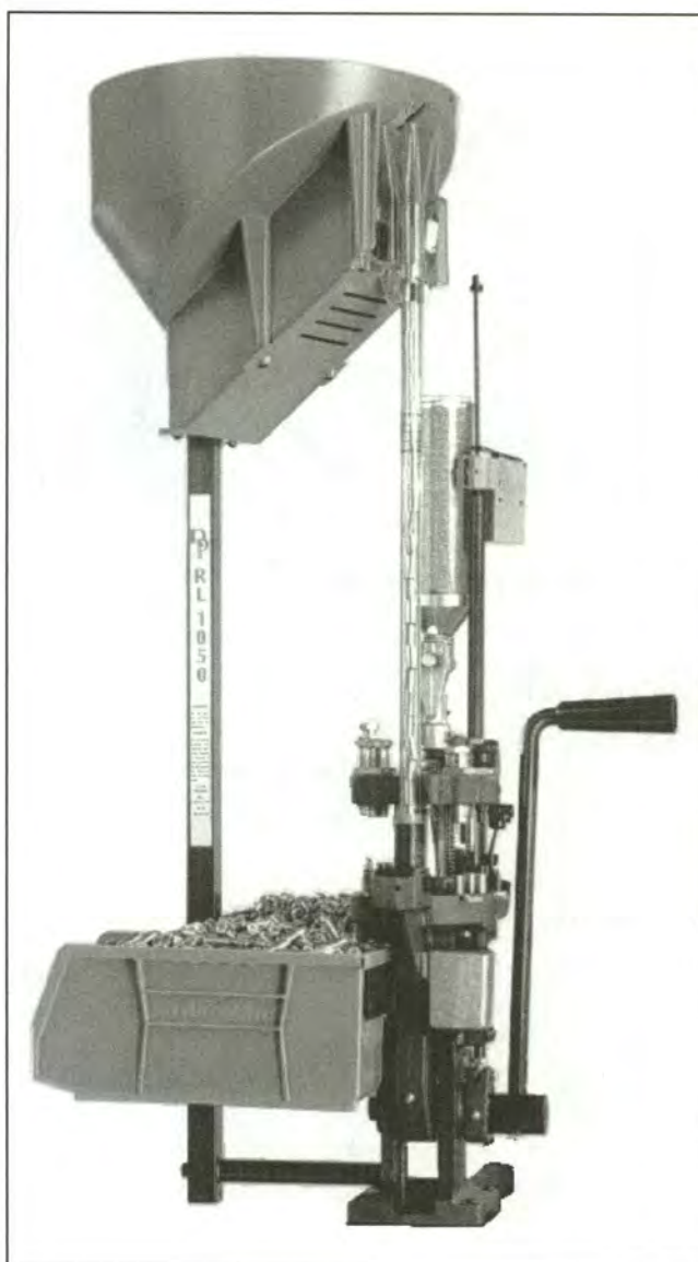
The Dillon RL 1050 will load 1000 to 1200 rounds per hour. A progressive loader of this sort represents a sizable investment and is definitely not for beginners.
