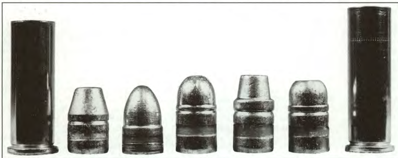
38-calibers reign. (From left): a 38 Special case, a 125-grain FP and RN, 158-grain RNFP, SWC, and RN, and a 357 Magnum case.
