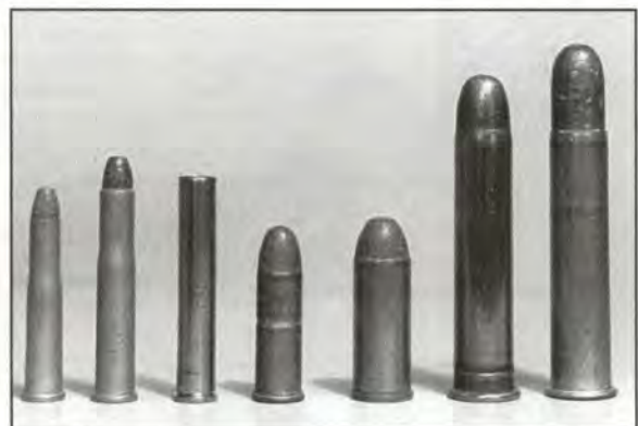
Old copper and soft brass cases from the last century and the early part of this one are a bad bet for reloading. They are often corroded by the blackpowder they contained, by deterioration through exposure to pollutants, or are simply made of poor metal and are too weak for modern smokeless pressures. Examples include, left to right: 22 WCF, 25-20 SS (with a newly-made 25-20 case), 38 Long, 45 S&W, and two 45-70s.
