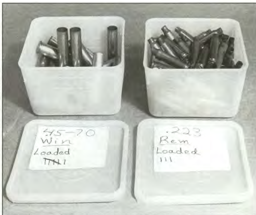
Plastic boxes are good for case storage and do a good job of keeping moisture and pollutants out if they're closed on a dry day and kept closed. The cases should always be identified by maker, caliber and number of times reloaded.
