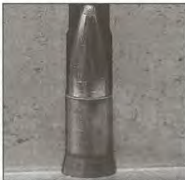
Cutaway neck and throat section of a bull barrel chambered for a 22-caliber centerfire varmint cartridge. For safety's sake, the case neck must have at least minimal clearance when chambered.
