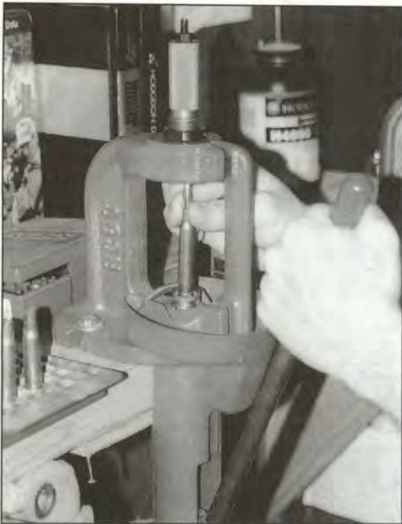
After the case is primed and powder added, author loads rifle cases one a time in this single-stage press.
