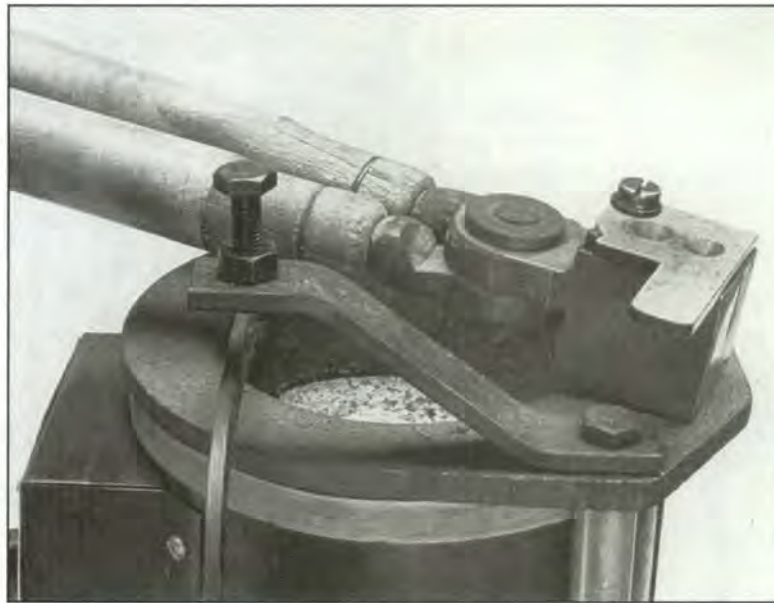
Bullet moulds can be warmed by placing them (carefully) on the edge of the melting pot. A pre-warmed mould will start producing good bullets before a cold one.
