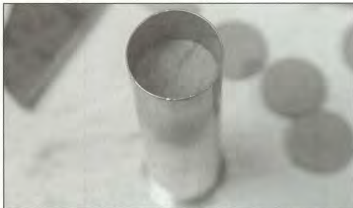
45-70 Govt. case loaded with 60 grains of Goex Cartridge and a fiber wad atop the charge. The thin card wad protects the bullet base but may not be necessary for hunting loads.
