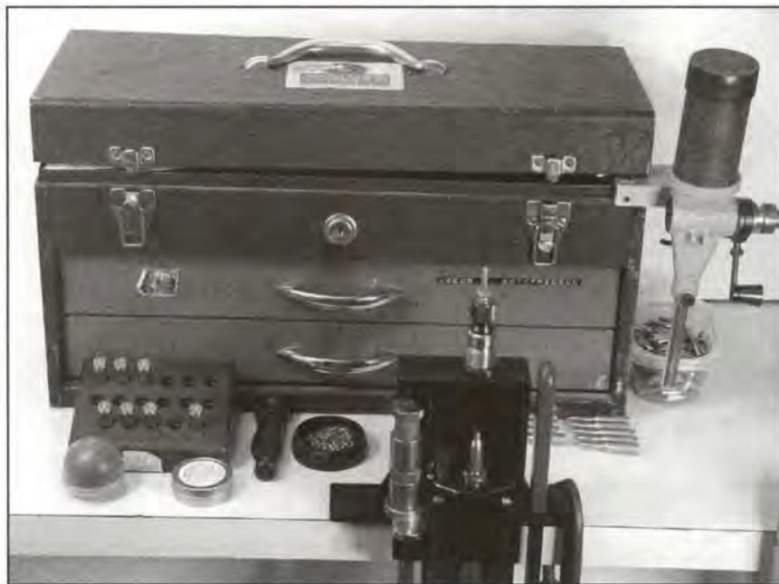
A rather old, but typical, match reloading bench. The loading box in the background holds all the tools necessary for loading at a match. The press in the foreground is manufactured by Hood and is made to fit in loading boxes like the one shown. The sizing die in the press is custom made to just bump the shoulder, decap, and size the body approximately .001-inch to allow fast feeding in the action. The seating die on the left is a Wilson Straight Line Seater. On the far left are a Crazy Kloth to clean the case, a cartridge block with spent cases, Imperial Die Wax, a K&M primer seater, and primers. The powder thrower is an original Culver measure with a drop tube installed, behind which are match bullets. This bench is ready to reload cases for competition.
