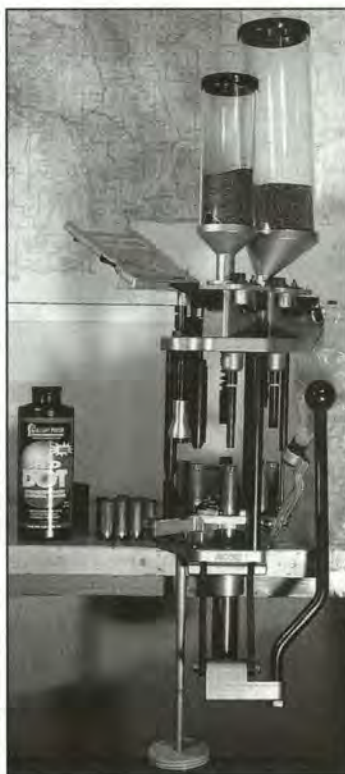
RCBS Grand. Every pull of the handle kicks out another completed shell.
