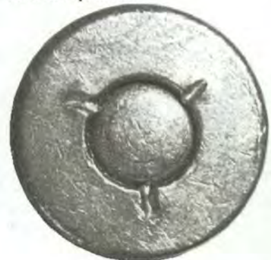
(Above and below) Military ammunition generally has the primer swaged in the case with a primer crimp, which makes first-time removal a little difficult. Once the crimp is removed, however, there is no further problem.
