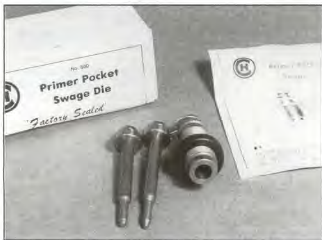
Primer crimps are easily removed with this handy tool (and others), which also swages the primer pockets to uniform size.
