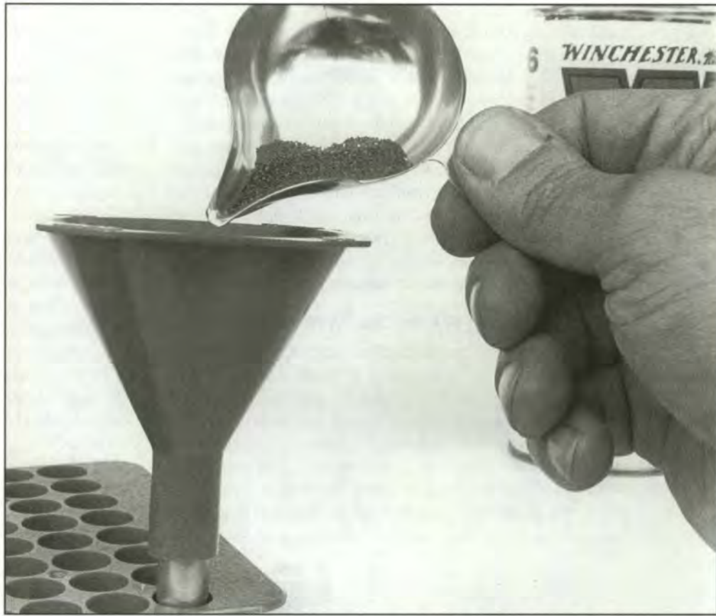
The reloader's powder funnel is especially designed to fit over the case mouth and deliver powder without spills.
