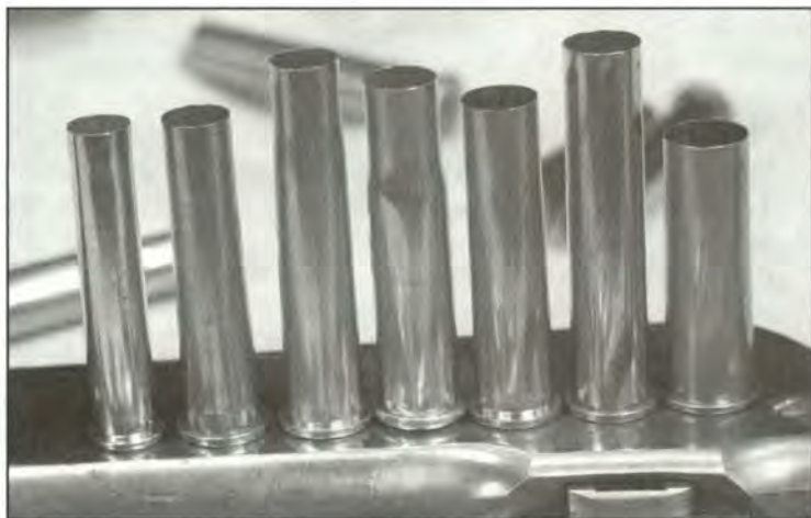
Brass is available for almost any obsolete blackpowder cartridge. Cases shown (l-r) are 38-55 by Winchester, 40-65 by Starline, 40-82 and 43 Spanish by Buffalo Arms, 45-70 by Remington, 45-90 by Starline, and 50-70 Govt. by Bell.
