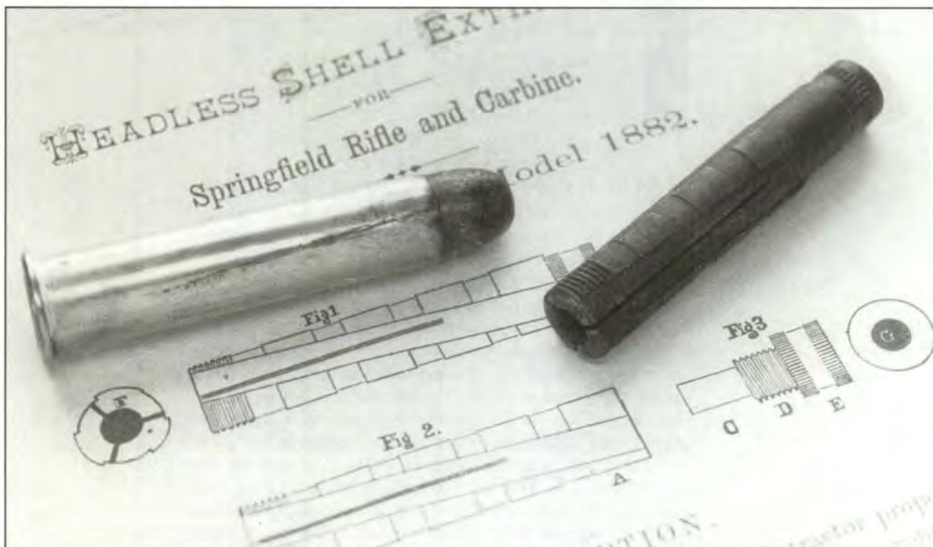
In the last century, the headless shell extractor was a necessary part of the shooter's kit, given the poor quality of the cartridge cases.
