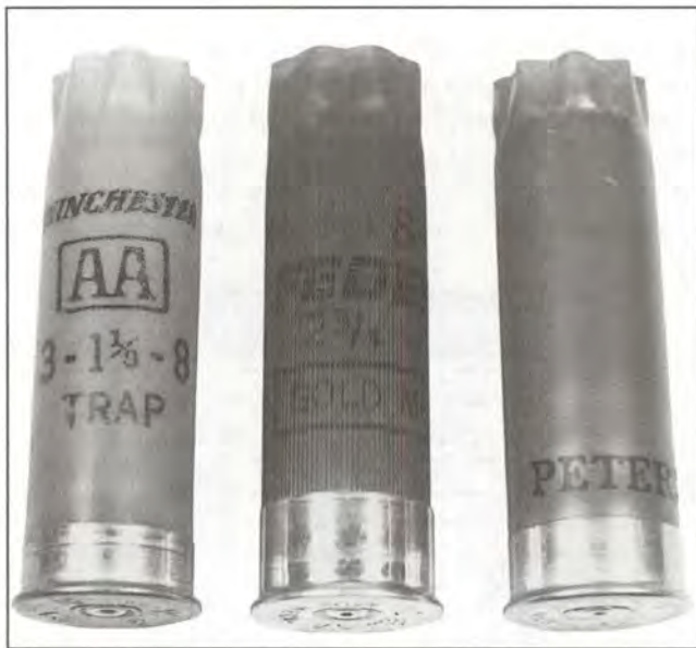
While steel shot can be reloaded in the same hulls used for reloading lead, the increased capacity of hulls such as the Federal Gold Medal plastic hull (center) are the best for reloading steel.
