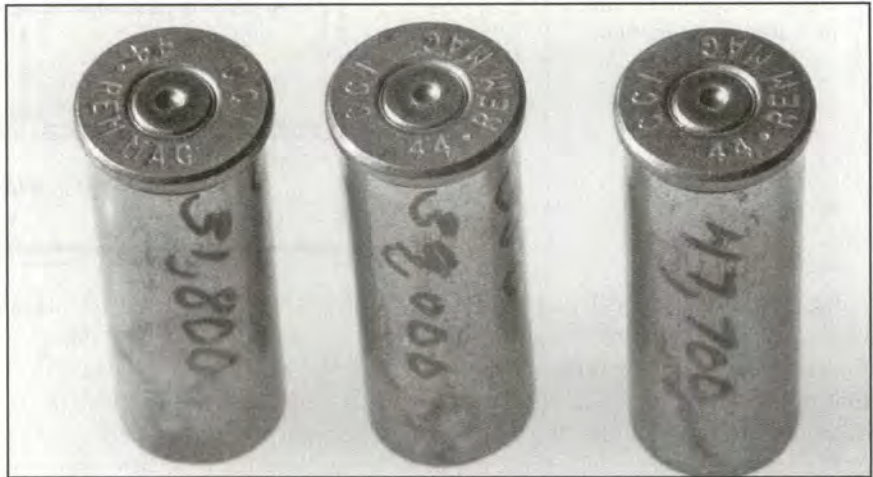
These three 44 Magnum cartridges were fired under the same conditions with the pressure measured by a copper crusher. Left to right: 31,800 CUP, 39,000 CUP, and 47,700 CUP. As can be seen, there is no discernible difference! (Photo courtesy Speer.)
