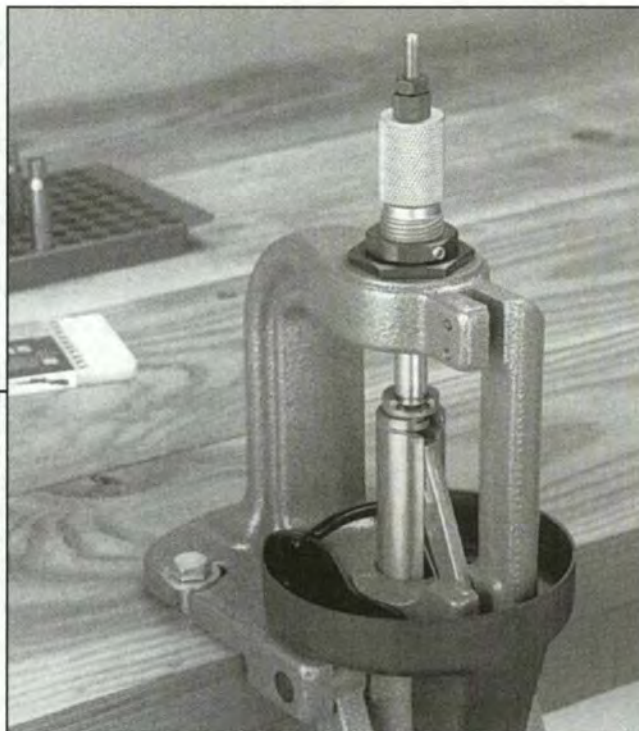
Step 11 - Priming (C): Gently and slowly raise the press handle. This lowers the case onto the priming arm, seating the fresh primer. Check each case to be sure the primer is fully seated.
