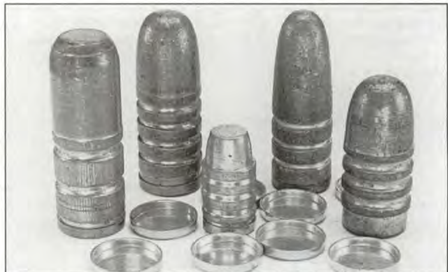
Copper gas checks applied to bullets designed for them will allow increased velocities and keep hot gas from melting the bullet bases.
