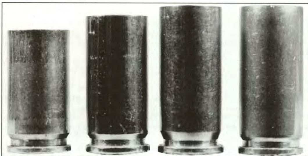
9mm cases – the long and short of it. (From left): the 9mm Luger, 9x21, 38 Super, and 9x23 Winchester.
