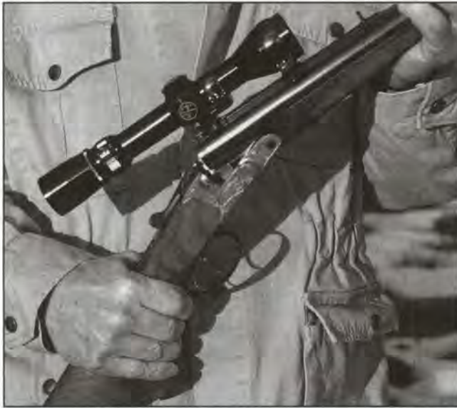
Some experienced African hunters prefer a double rifle to a bolt action for the speed of the second shot. Rifle shown is author's Krieghoff side-by-side 375 H&H flanged, with quick-detachable scope mounts and fixed iron sights.
