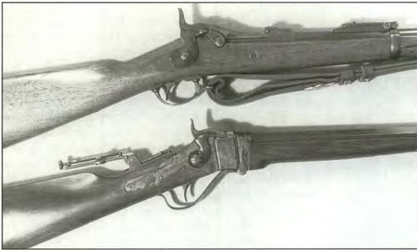
This reproduction 1874 Sharps rifle ( bottom ) is made of modern steel (4140 for the receiver and 1195 for the barrel). It is capable of handling modern high-pressure 45-70 loadings to 28,000 psi. The Allin "trapdoor" 45-70 Springfield ( top ) was made in 1888. The receiver is mild steel, casehardened. The barrel is mild "decarbonized" steel. Its maximum pressure rating, at the time of manufacture, was 25,000 psi. It is not a modern gun and must be loaded accordingly.
