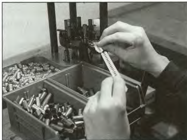
APS strips feed into the Piggyback 4 progressive press. Strips link together to keep the loading process going without interruption.
