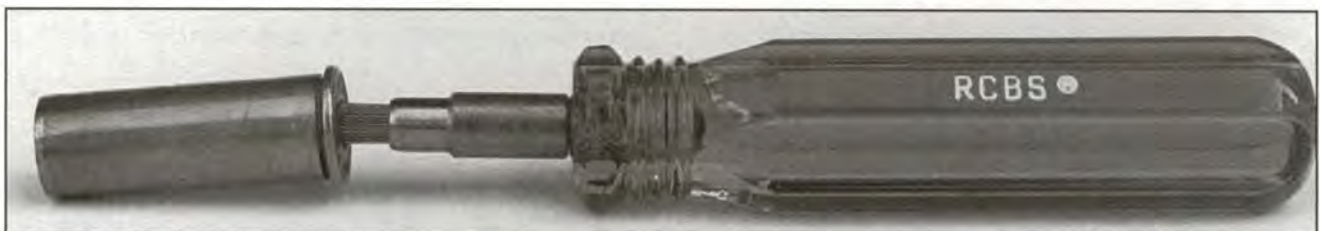
Primer pocket cleaners scour burned residue from the primer pocket. This brush-type tool works quickly.
