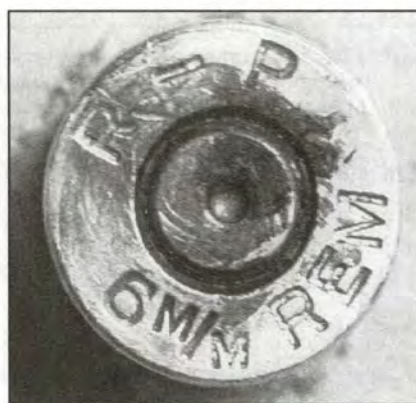
Primer pockets will stretch, as did the one on the left after a number of heavy loads. If the leak or stretch appears suddenly on a new or nearly new case, you are in the very high pressure range and should reduce your loads.
