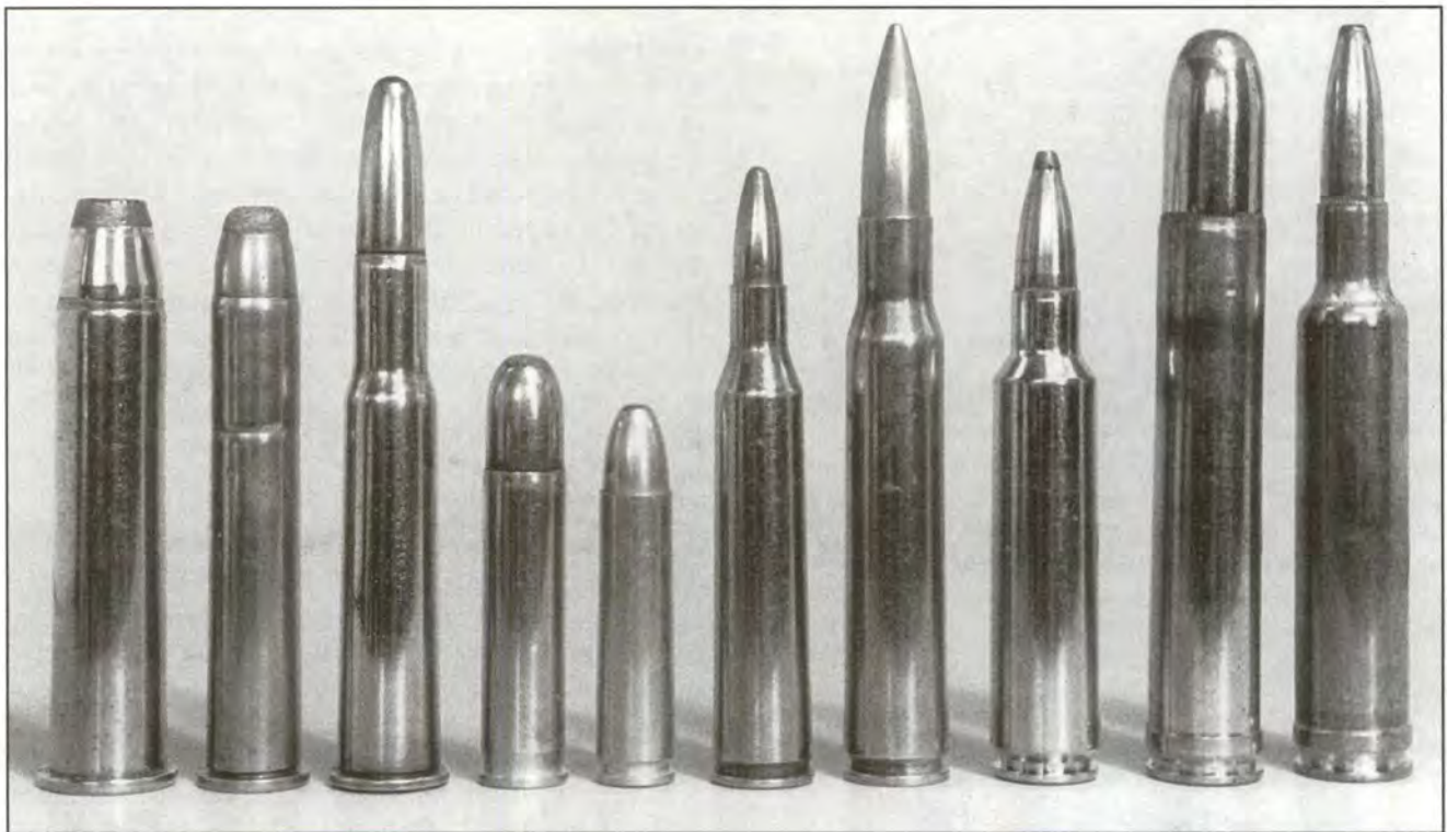
(Above) Basic cartridge case forms include the following variations, left to right: straight-walled rimmed (45-70), straight-tapered (38-55), rimmed bottleneck (30-40 Krag), semi-rimmed straight (351 Winchester SL), rimless straight (30 Carbine), semi-rimmed bottleneck (220 Swift), rimless bottleneck (30-06), rebated head (284 Winchester), straight belted (458 Winchester Magnum) and bottleneck belted (7mm Weatherby Magnum).
