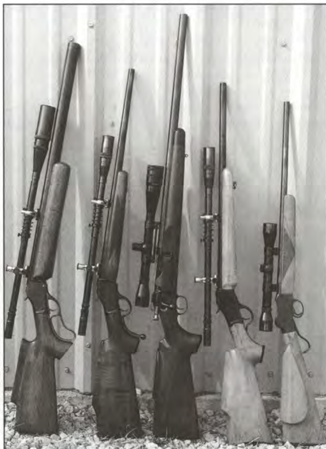
Some older varmint rifles used by the author (left to right): Winchester High Wall 219 Zipper w/12x Unertl, Winchester High Wall 219 Zipper w/10x Unertl, Krag-actioned 219 Zipper w/10x Lyman, Winchester High Wall 22 Hornet w/8x Unertl, BSA Martini 22 Hornet w/4x Weaver.
