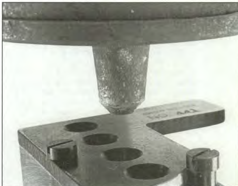
Best casting results can be had by holding the mould about an inch below the spigot rather than having it in hard contact.
