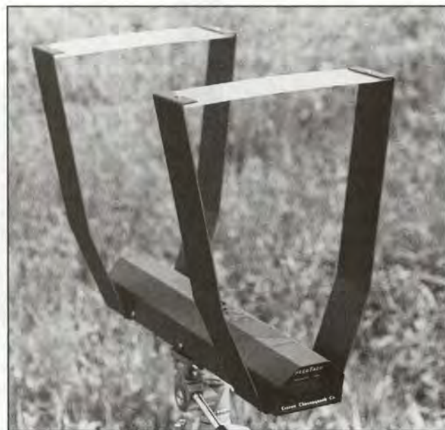
There is certainly nothing wrong with a chronograph that has the entire unit ahead of the shooter, but utmost care is necessary to keep from destroying the instrument with an errant bullet. Chronograph pictured is a SpeedTach by Custom Chronograph Co. that the author used in the mid-'80s.
