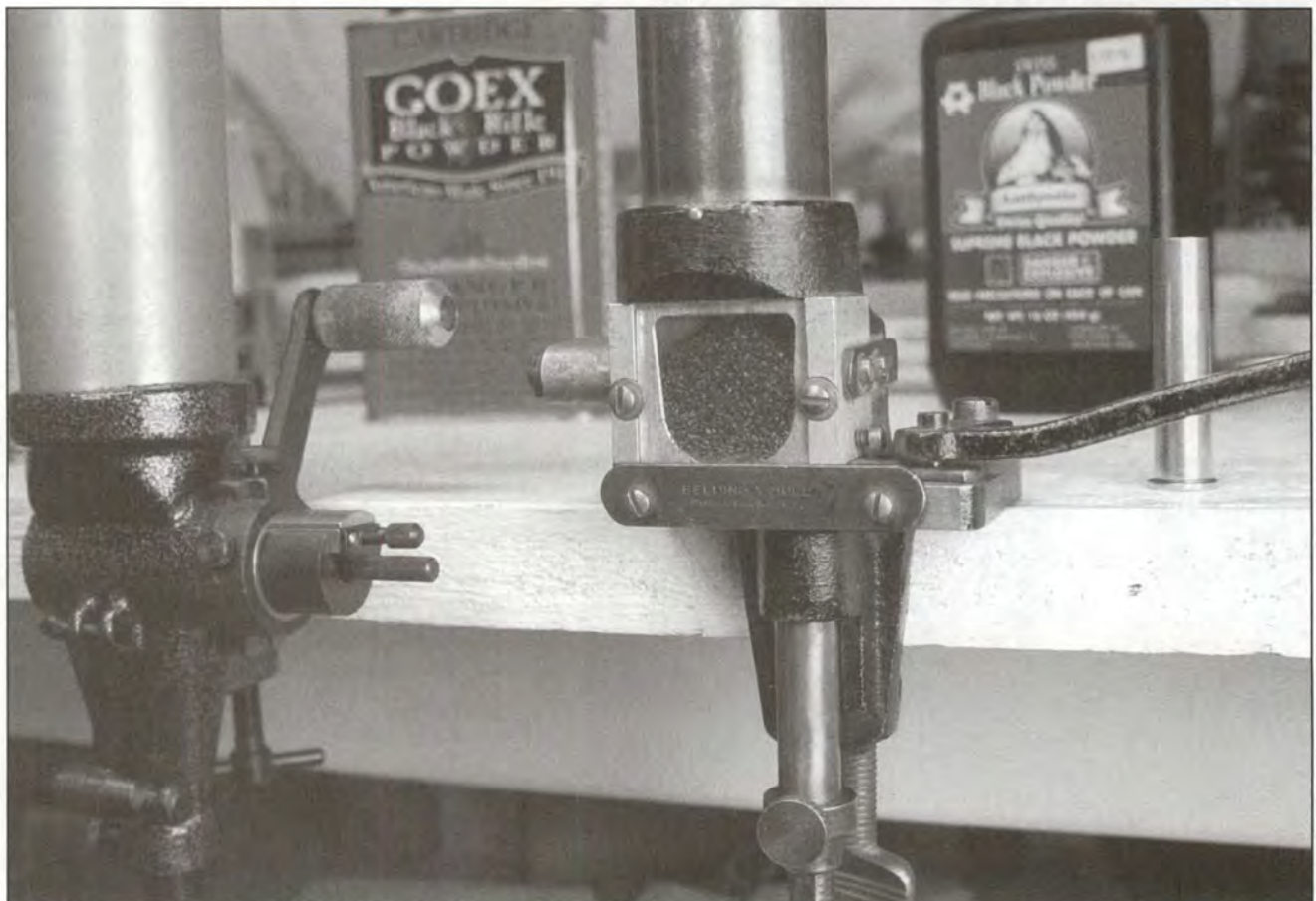
Powder measures for metering blackpowder, Lyman 55 Blackpowder Measure ( left ) complete with drop tube (not seen) and a vintage Belding & Mull Visible Powder Measure ( right ).
