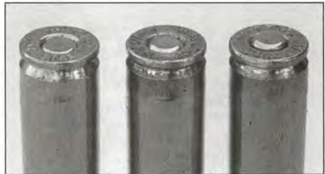
(Below) Pistol primers should not be used in rifle cases since they will seat too deeply, as in the case on the left. The center case shows proper seating depth, while the high primer on the right will give poor ignition and possibly slam-fire in an autoloader.
