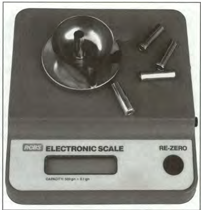
Sorting cases by weight is the traditional method for ensuring consistent results.
