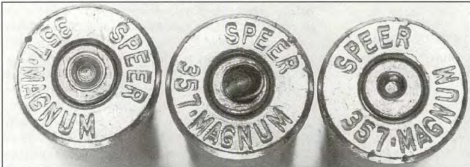
The cratered primer (center) appears at first glance to be evidence of excessive pressure. The actual cause was an oversize firing pin hole and a soft primer.
