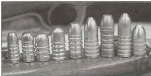
Blackpowder hunting bullets should have a flat point or large round nose with many grooves for carrying lots of lube. Shown are bullets in 38-, 40-, 45-, & 50-caliber from bullet moulds by Lyman, RCBS, SAECO, and custom mould maker Steve Brooks.
