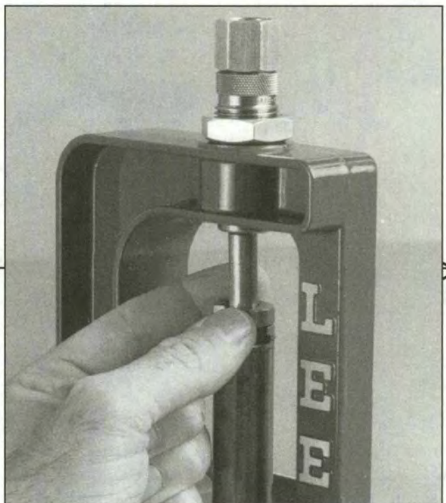
Step 7 - Case Mouth Expansion: After installing and properly adjusting the expander die, insert a case and run it into the die to bell the case mouth for easy insertion of a new bullet. Adjust the die just enough to allow easy bullet entry.
