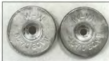
The flash hole on the case at the left was deliberately enlarged to burn a compressed blackpowder load. If this case were loaded with smokeless powder, dangerously high pressures probably would be generated.
