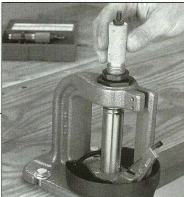
Step 15 - Bullet Seating (A): Thread the seater die into the press a few turns. With a case in the shellholder, lower the press handle, running the case all the way up into the die. Turn the die further in until it stops. While using the headstamp on top of the die as a reference, back the die out one full turn and lock it in place with the lock ring.
