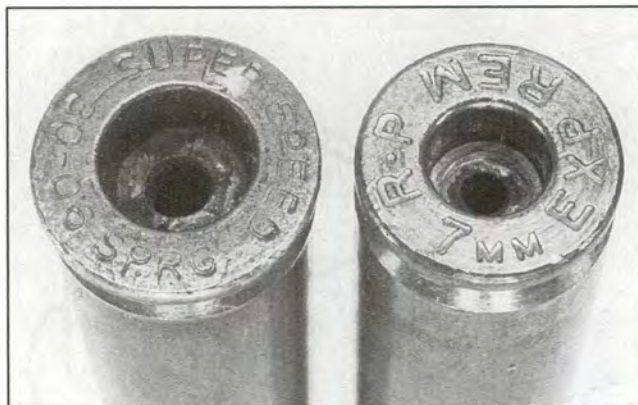
Primer pockets will stretch, as did the one on the left after a number of heavy loads. If the leak or stretch appears suddenly on a new or nearly new case, you are in the very high pressure range and should reduce your loads.
