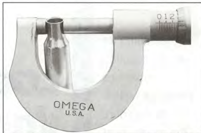
The micrometer is indispensable for the serious handloader, here measuring case neck thickness.
