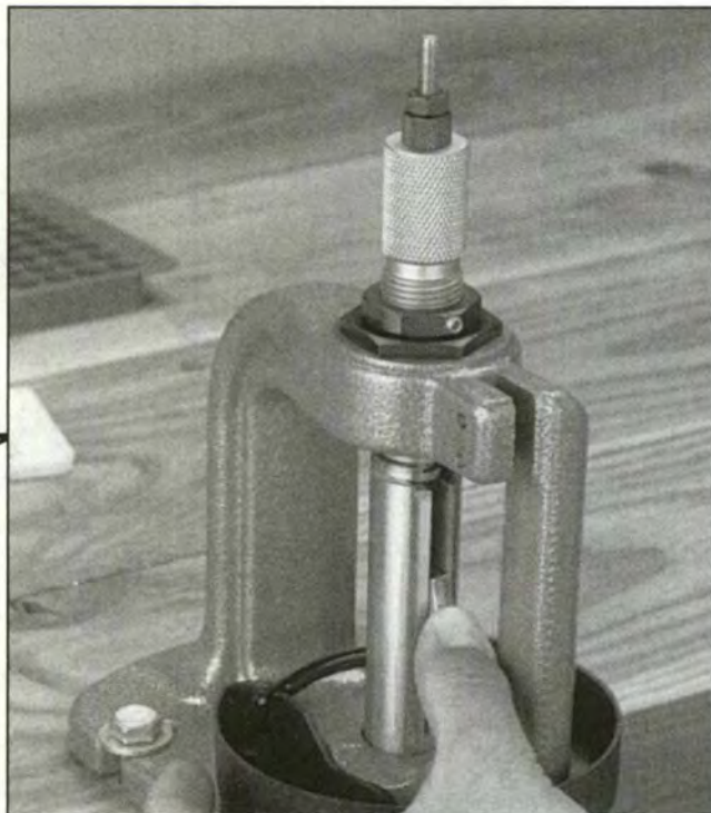
Step 10 - Priming (B): Lower the press handle and push the primer arm all the way into the slot in the ram.
