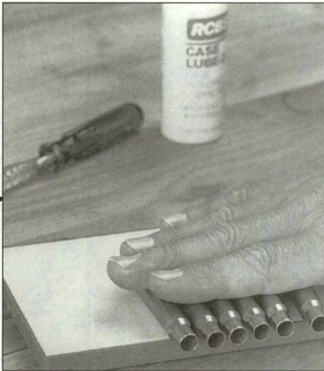
Step 2 - Lubricate the Cases: To prevent the case from sticking in the sizing die, it must be lubricated only with sizing die lube. With a bit of lube on the pad, roll a number of cases over it a few times to lightly coat the case body.
