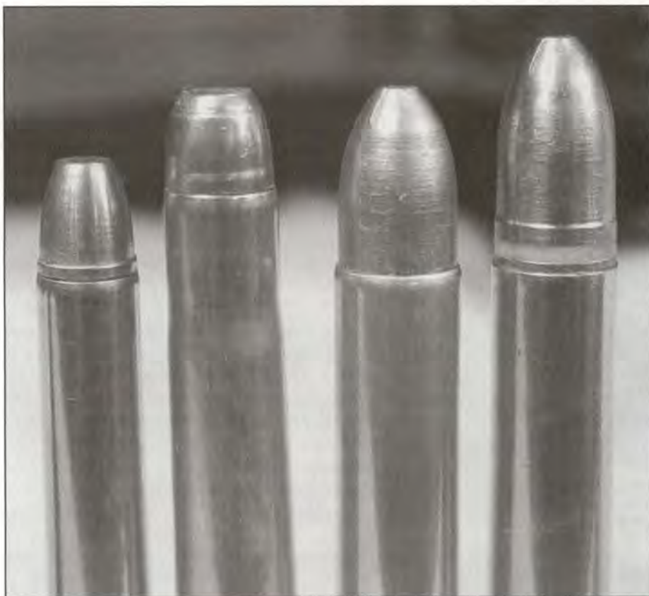
Finished blackpowder loads having varying degrees of crimp: (l-r) light, moderate, heavy, and none. Of the two 45-70 rounds on the right, the left one is our test example having the case mouth crimped over the front driving band. The one on the right utilizes the same bullet seated shallower with a heavier powder charge, and not crimped.
