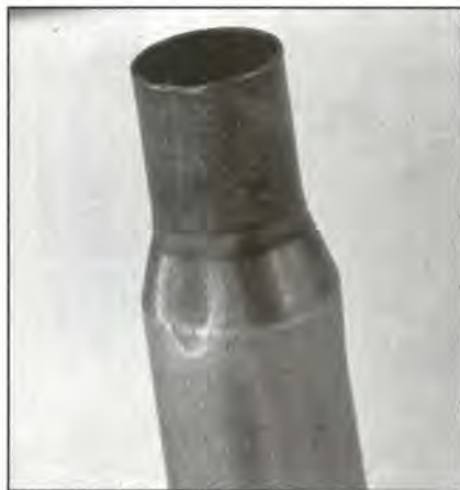
Too much lubricant will make dents in cases. These will flatten out on firing, but this works and weakens the brass.
