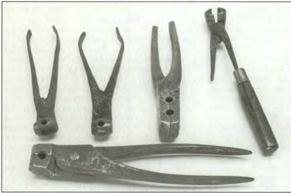
Bullet moulds from the late 18th and early 19th century cast round balls and roughly shaped conical bullets. Most had metal handles that heated up right along with the mould blocks. The finished bullet was trimmed up with a pocketknife.
