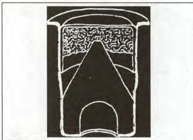
The shotshell battery cup primer comes with the primer pocket and vent as part of the unit, all of which is replaced when the shell is reprimed.
