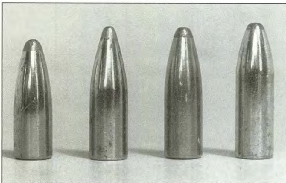
Bullets for the 22 centerfire (from left): 55-, 60-, 63- and 70-grain. They look very alike and can be easily mixed up, which is why unloaded bullets should always be returned to the original container after you are through loading ammunition. The 70-grain bullet will not work well in slow-twist (1:14-inch) barrels.
