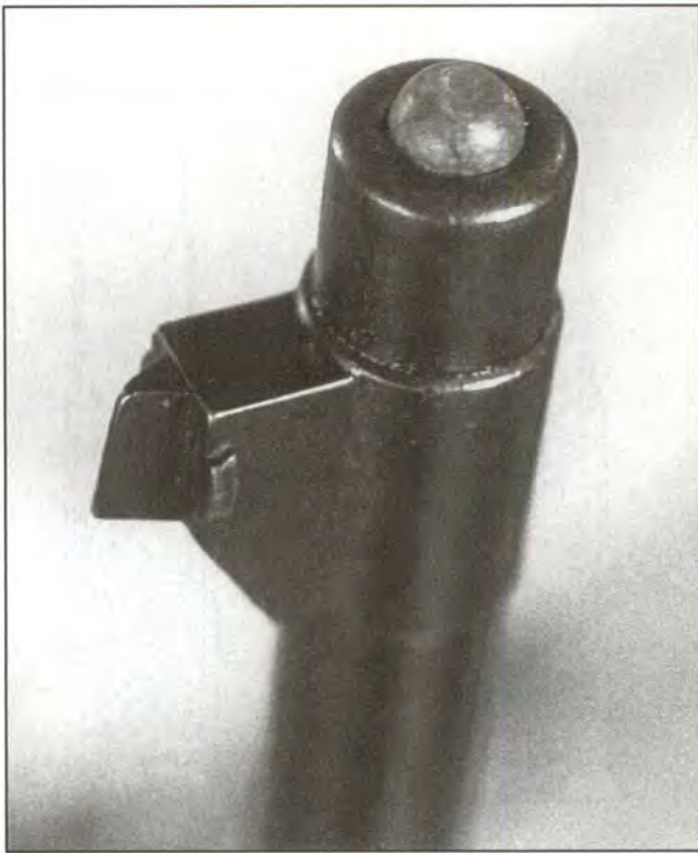
(Above and right) Slugging the bore consists of carefully driving a small, soft pure lead slug down the barrel. If done from both ends, the two slugs can be compared for tight and loose spots in the barrel.
