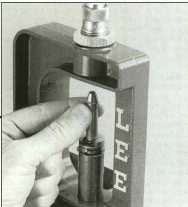
Step 14 - Bullet Seating (C): To seat a bullet, place one in the case mouth and guide it into the seating die as straight as possible. If the bullet needs to be deeper, screw in the seater plug a little bit and run the case back into the die. It may take a few tries to get the exact depth required.
