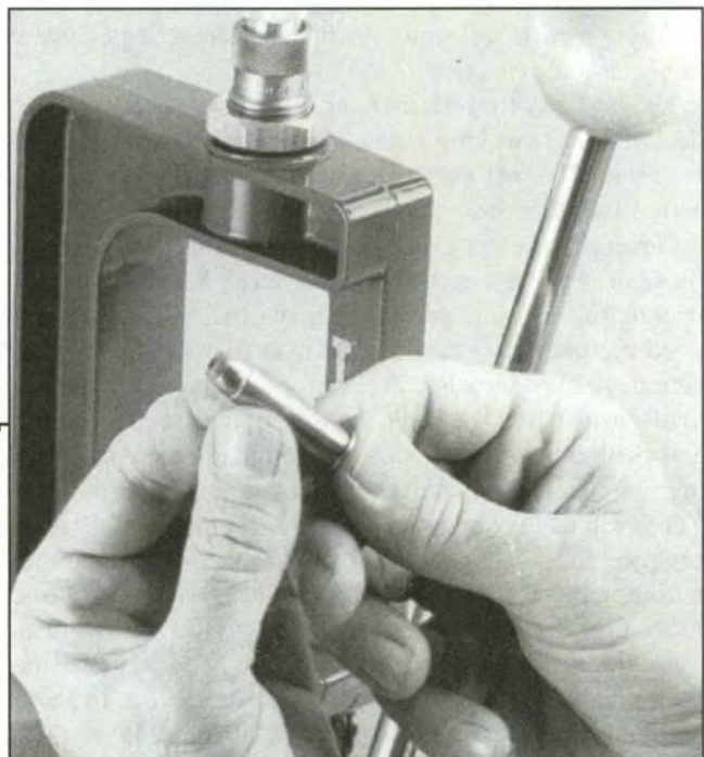
Step 15 - The Loaded Round: That's all there is to loading a handgun cartridge. A final wipe with a clean cloth and the ammunition is ready to be fired. Don't forget to mark the ammo box with your load data so you can repeat the load.
