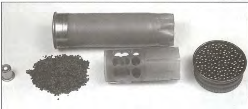
Steel reloading is much like reloading lead shot target loads in that only a hull, primer, powder, wad and shot are needed as components. Unlike the lead wad pictured here, however, a steel shot wad does not contain cushioning posts, is molded from a much higher density plastic, and contains a much deeper shotcup.
