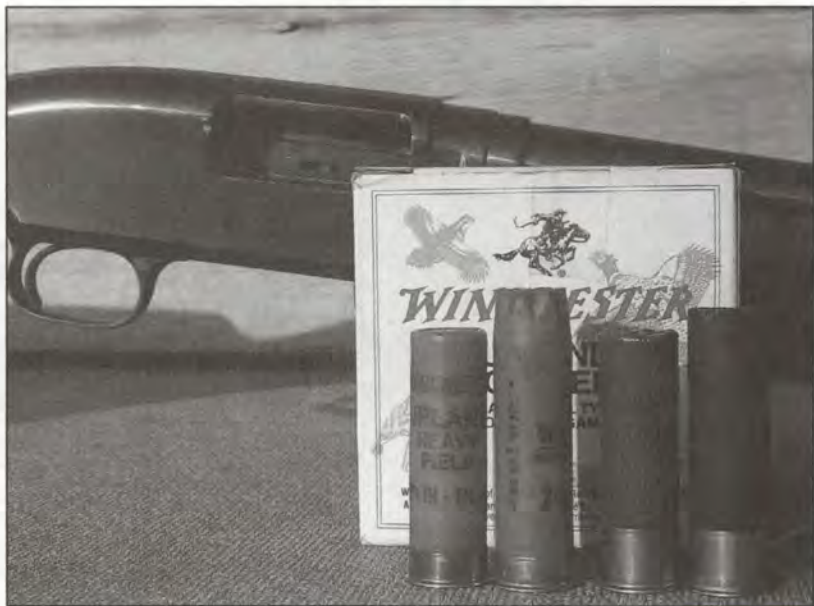
Snipping off 16-gauge shells to 2-9/16 inches, and then loading them, gets my old Model 12 16-gauge up and shooting.
