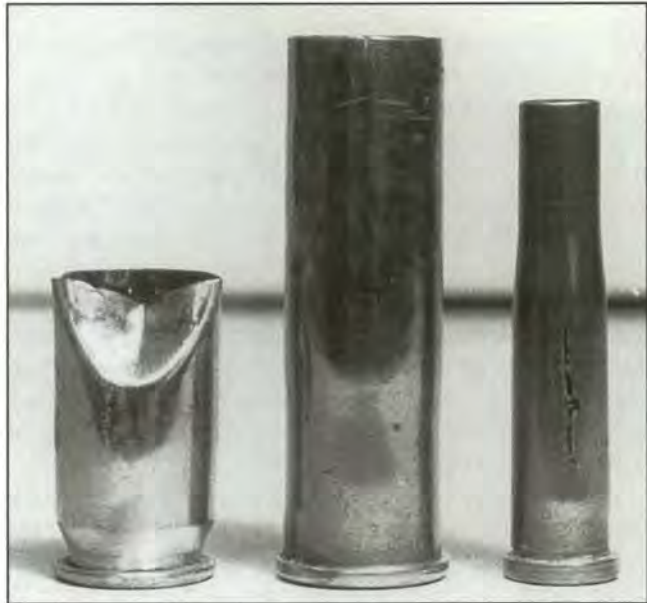
This 45 ACP has been so badly battered that it will probably not go into the resizing die. The split in the body of the 22 Hornet probably resulted from too many reloadings. The tiny split on the mouth of the 44 Winchester (center) could be easily overlooked. All are rejects.
