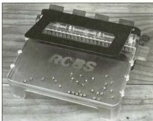
(Left and above) Primers are sold preloaded in strips, but the strips can be refilled with the RCBS loading tool. You have to buy the system. (Photos courtesy RCBS)
