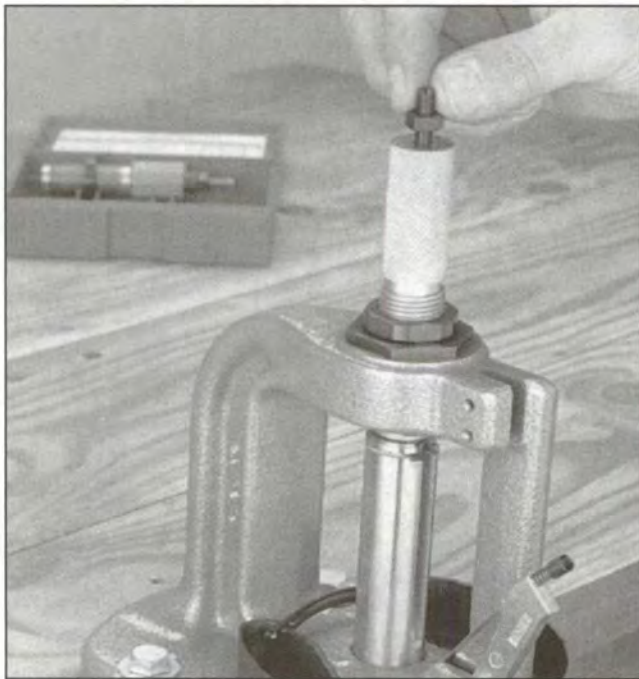
Step 18 - Bullet Seating (D): If the bullet needs to be seated deeper into the case, turn the seater plug down a little and run the case back up into the die. Make small adjustments and keep trying and measuring until you get the proper cartridge overall length. Once the proper setting is reached, tighten the seater plug lock ring.
