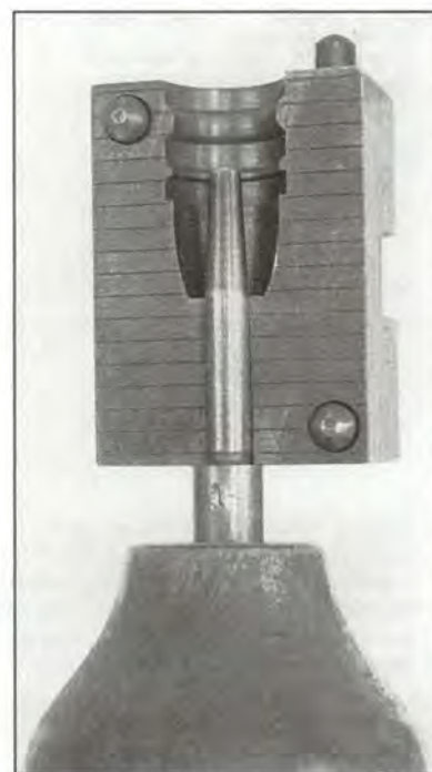
This hollowpoint plug fits into the nose end of a base-pour mould.
