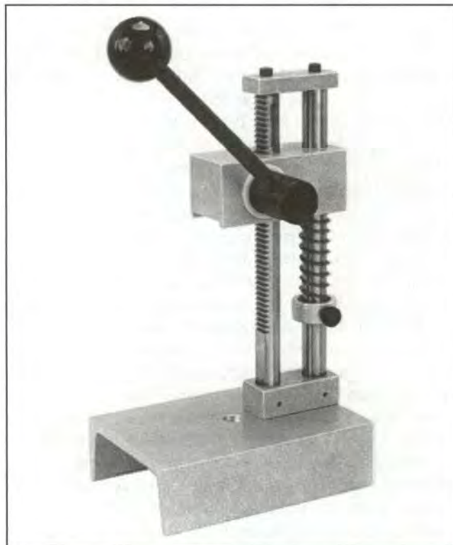
The Jones arbor press is typical of the type. Arbor presses are compact and do not need to be bench-mounted, making them convenient to take to the range to assemble ammunition on the spot.
