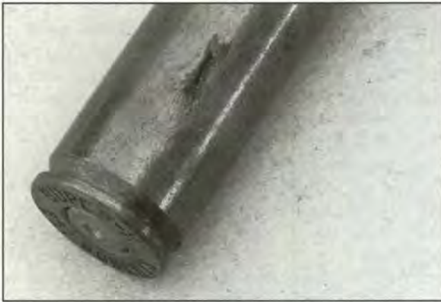
Case failures are not common, but they do happen. The nearer to the case head the rupture, the more serious it is.
