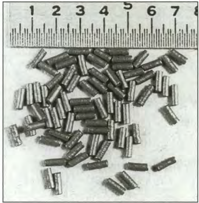
IMR 3031 powder is an extruded single-base propellant made of nitrocellulose. It has a fairly slow burning rate and has long been a standard for military rifle cartridges.
