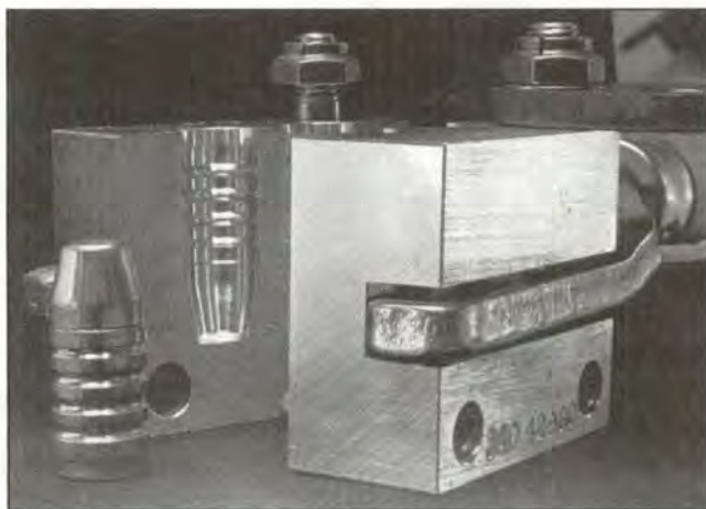
Aluminum moulds do not require as much breaking-in as iron or steel moulds. However, the cavity must often be coated with either carbon smoke or a special compound to get good bullets.
