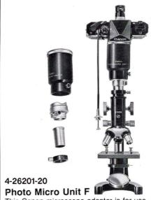
This Canon microscope adapter is for use where a fixed camera-to-microscope distance is acceptable. It is suitable for photography with general and metallographical microscopes with a 25mm diameter outside sleeve. Magnification is approximately 0.5X that of the microscope eyepiece objective.
